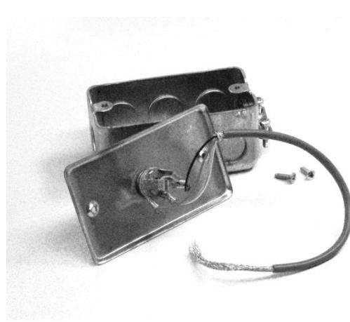
The splice point should stay inside the junction box. That is, you want to feed the long run of data cable into the box rather than pulling the pigtail out. Electro-Mech provides a strain relief on one side of the junction box to secure the cable. You may choose to connect conduit directly to the junction box, in which case the strain relief will not be needed. The junction box is designed to accept 3/4-inch conduit fittings.
