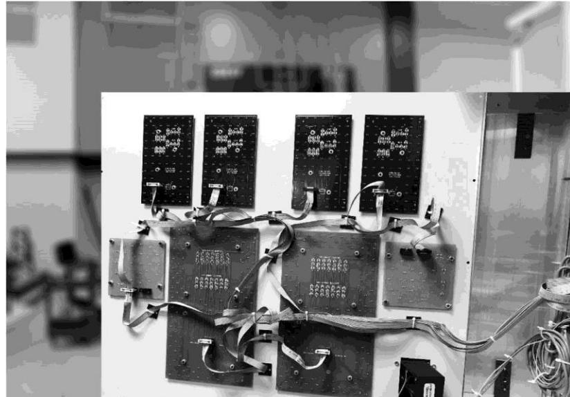
Each LED digit PCB is held to the face by several nuts, which you can remove using a 3/8-inch nut driver. Be careful to keep the PCBs right side up when you mount replacements behind the shot clock face.
