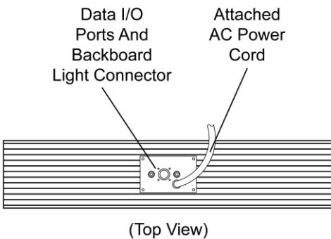
There are two common methods for bringing the last few feet of data cable to one of the shot clock displays. One method involves installing a junction box on the wall or other structure near the display. From here you can run a patch cable to the shot clock's data input port. The standard scoreboard package does not include extra junction boxes and patch cables for this type of cable routing.
